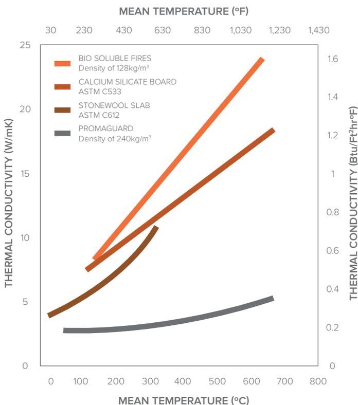
Third-party tests show how layers of Promaguard suppress thermal conductivity and delay the onset of a fire
